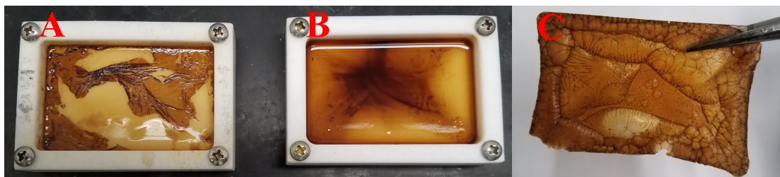
Figure 3.7 Solvent cast films of CL (5 wt%) and P(MA-co-AA) in (A,B) MeOH and (C) THF/H 2 O. Films differ by (A) 10% AA and (B,C) 20% AA copolymer content.
